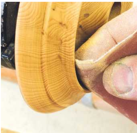
▲ Pic.16 When sanding the shape don't round over the edges. The main benefit of hand turning is that you can achieve really crisp edges that cannot be done on most automatic lathes
